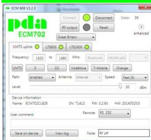
The operational parameters for the unit are programmed in using the special Windows. The two integral countermeasure units are programmed separately via the USB sockets on the front panel. When the PC is plugged into each unit the relevant operational options will be displayed.
